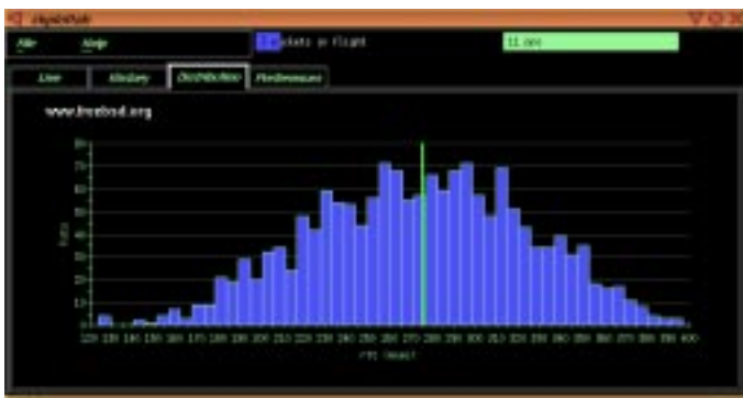
Figure 6: Histogram of RTTs for 1600 probes from lancelet.caida.org (in Ann Arbor, MI) to www.freebsd.org.
